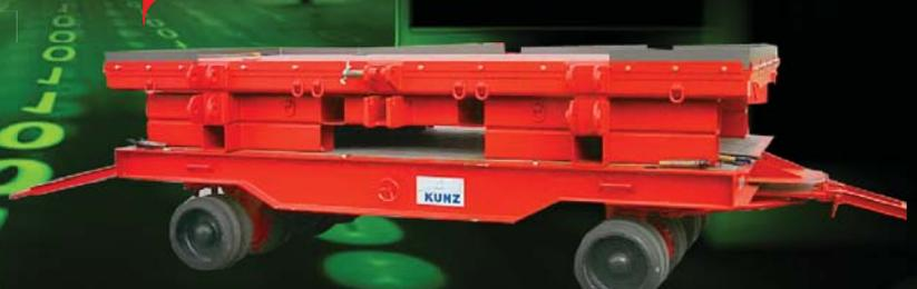
Disabled Aircraft Recovery Trailer are available in two sizes, 40 tonnes and 80 tonnes capacity to move narrow-bodied
