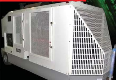
The Air Starter Unit series is a line of truck or trailer mounted continuous flow jet engine starting units
