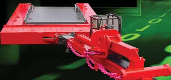
Aircraft Recovery Dollies for 'flat tires or damaged wheel' scenarios ensure rapid removal of an aircraft from runways.
