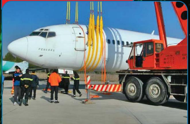
Lifting Sling Assemblies are used to lift disabled aircraft by means of lifting slings and cranes.
