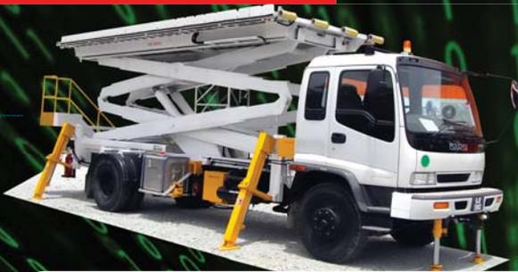
The Scissor Lift Maintenance Truck FHB-4.9 is designed for routine aircraft inspection and maintenance procedures
