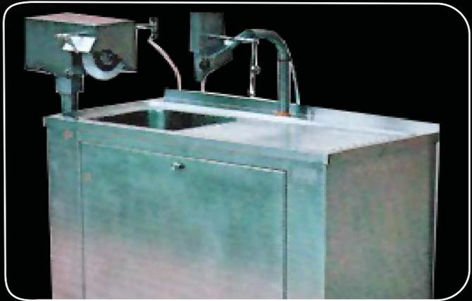
Auxiliary Gutting Device Cleaning System
